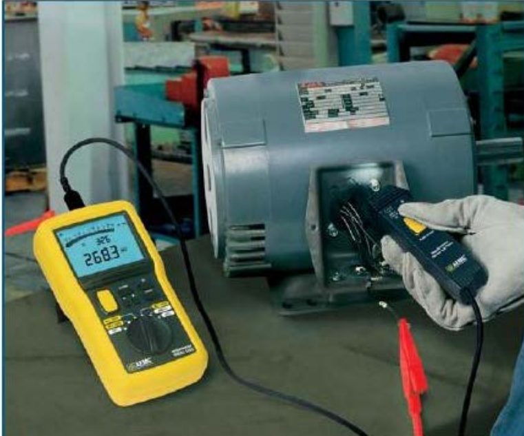
Figure 5.4 Motor Testing with a Megohmmeter. Source: www.aikencolon.com
