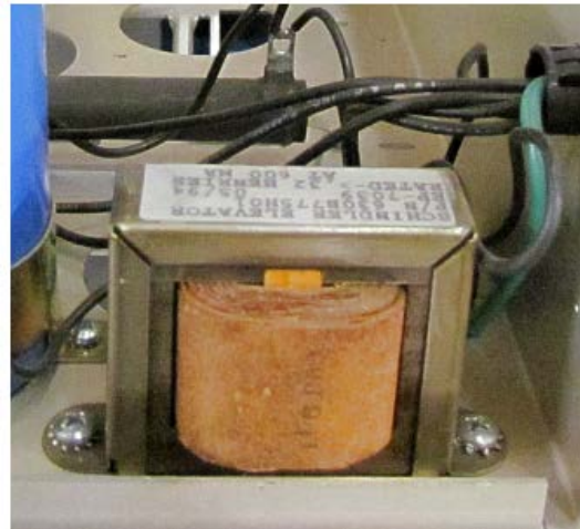
Figure 4.2 Step-Down Transformer 120 VAC to 36 VAC
